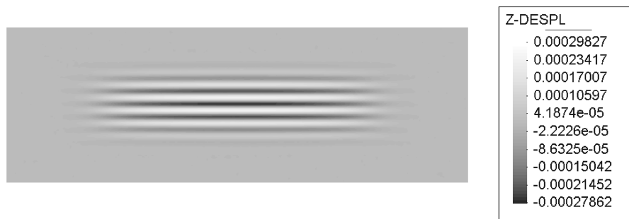
Fig. 10 Results of out-of-plane deformation of the membrane.
